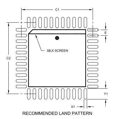
Units INCHES Dimension Limits MIN NOM MAX Contact Pitch Ε .050 BSC Contact Pad Spacing C1 .630 Contact Pad Spacing C2 .630 Contact Pad Width (X44) .026 Χ1 Y1 Contact Pad Length (X44) .094
